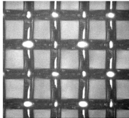
☀ Bulk Micromegas obtained by lamination of a woven grid on an anode with a photo-imageable film
