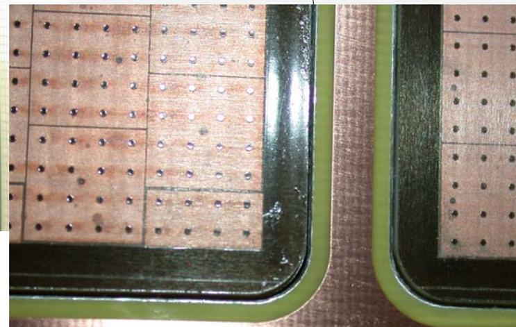
Inner surface covered by PCB for E-field termination
