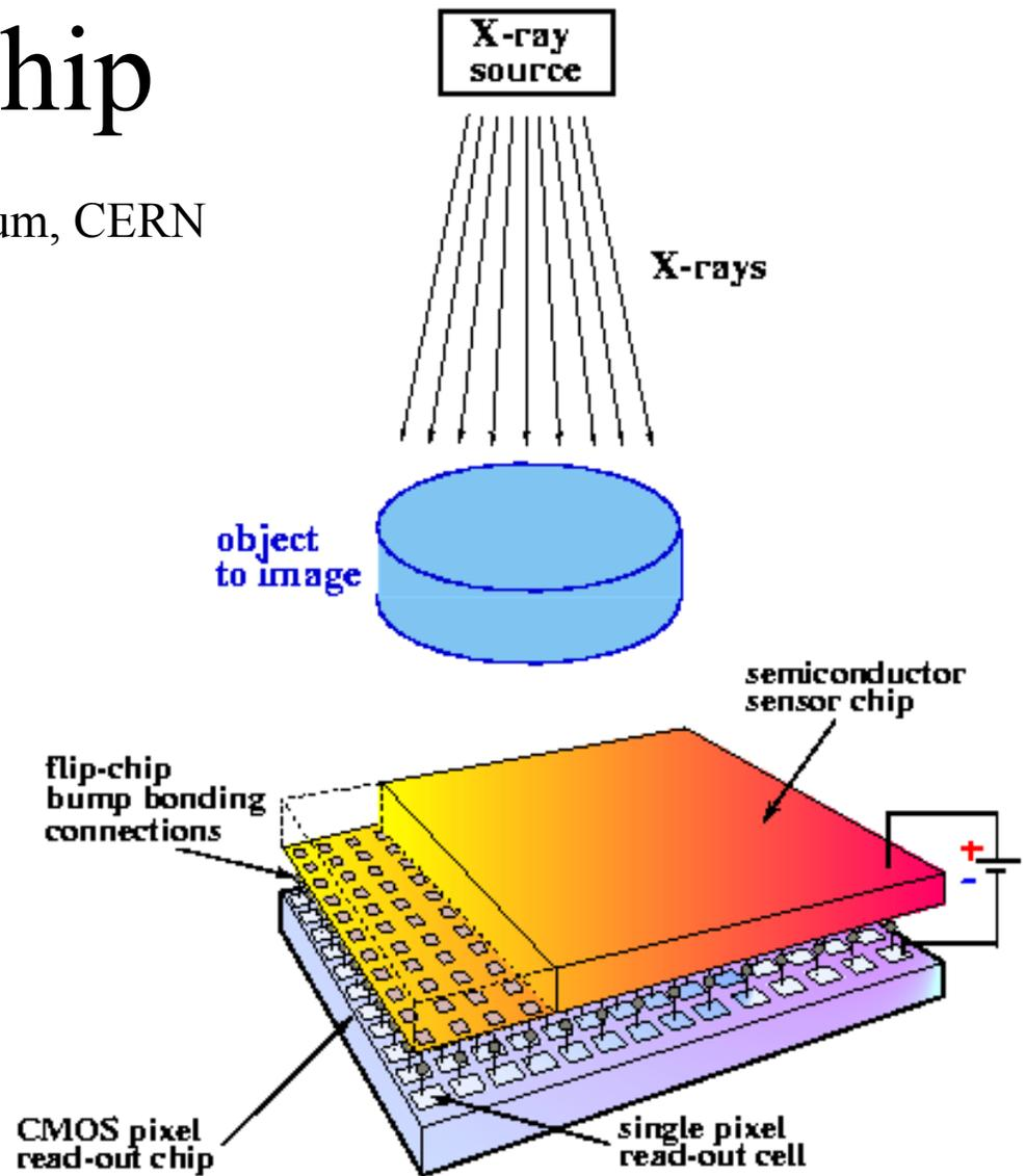
Use the “naked” chip as the detector anode
