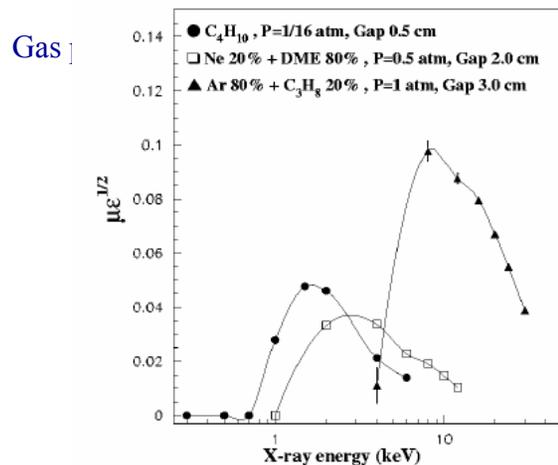
Polarimeter figure-of-merit vs energy
