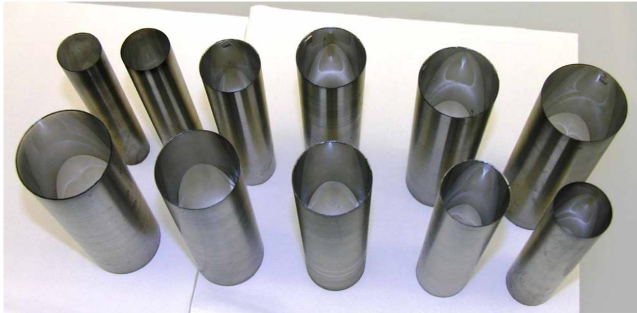
11 (out of 14) Ir-coated polycarbonate shells in LLNL cleanroom lab, prior to assembly
