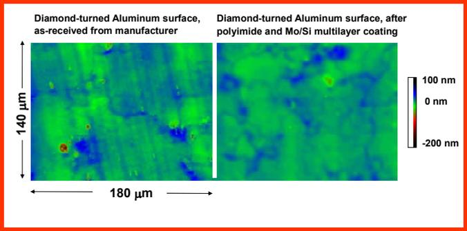
Measurements obtained with a Zygo New View™ optical profiling microscope operated at 40x objective lens magnification
