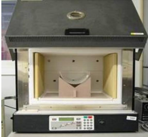
Slump 0.2mm-thick flat panel display glass in ovens
