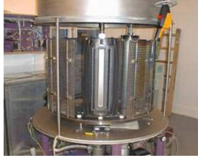
Coat glass with ~ few hundred layers (2.5-10nm each) of W/SiC, Pt/SiC to extend energy band
