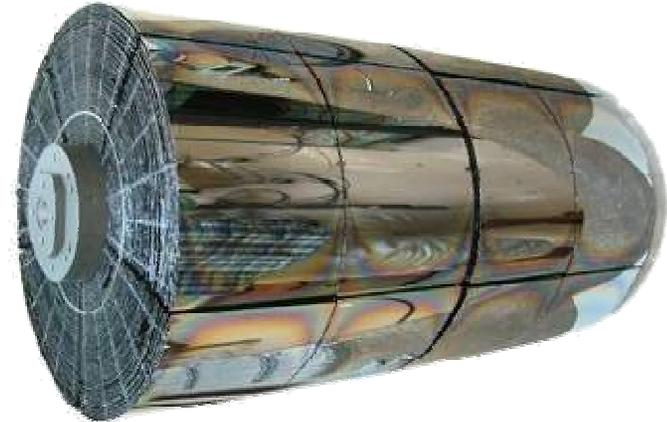
**A completed HEFT optic with 72 layers made up from 1440 individual mirrors (20-70 keV)**
