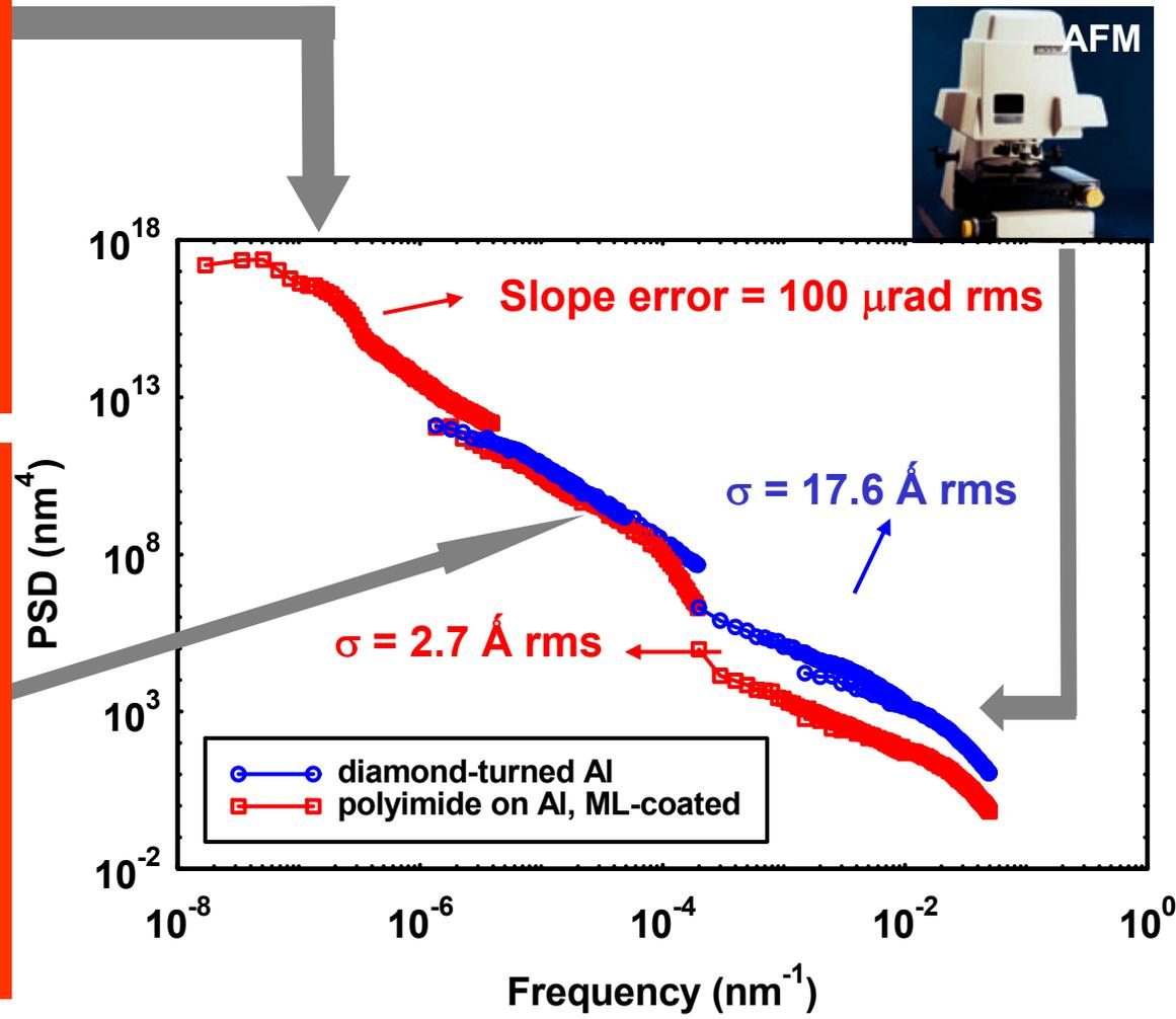
Polyimide smooths high spatial frequency roughness, including 10 μm-range diamond turning marks
