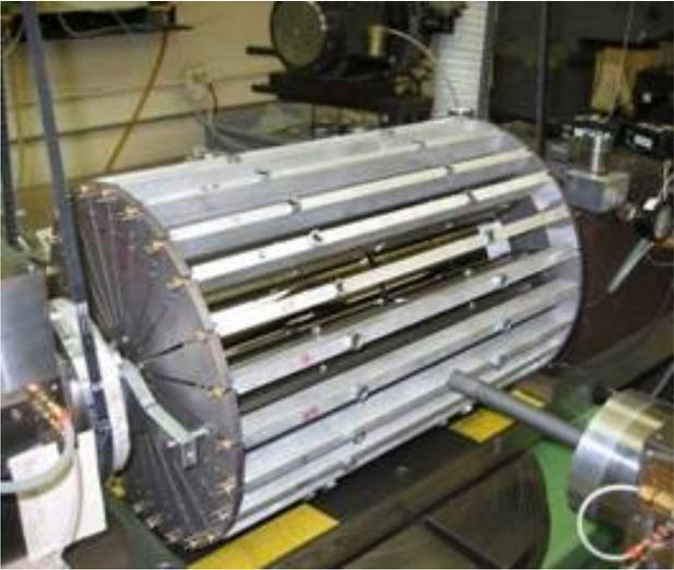
**Assemble the glass into an optic using graphite and epoxy.**
