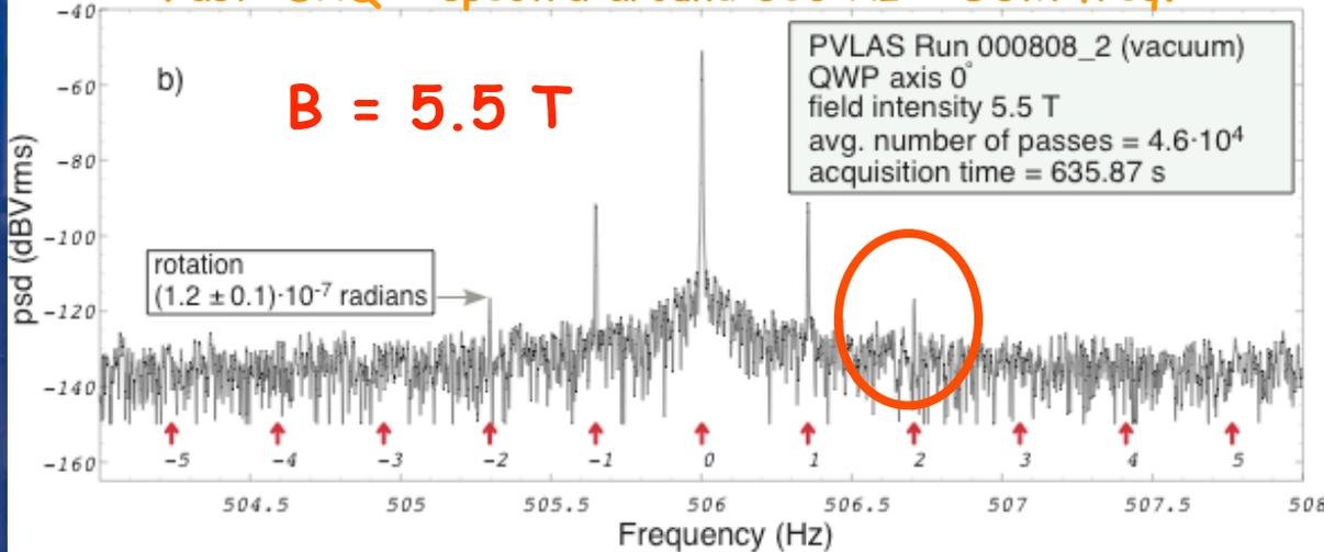
The rotation signal corresponds to a "true" rotation (dichroism) with amplitude  $(3.9 \pm 0.5) \times 10^{-12}$  rad/pass
